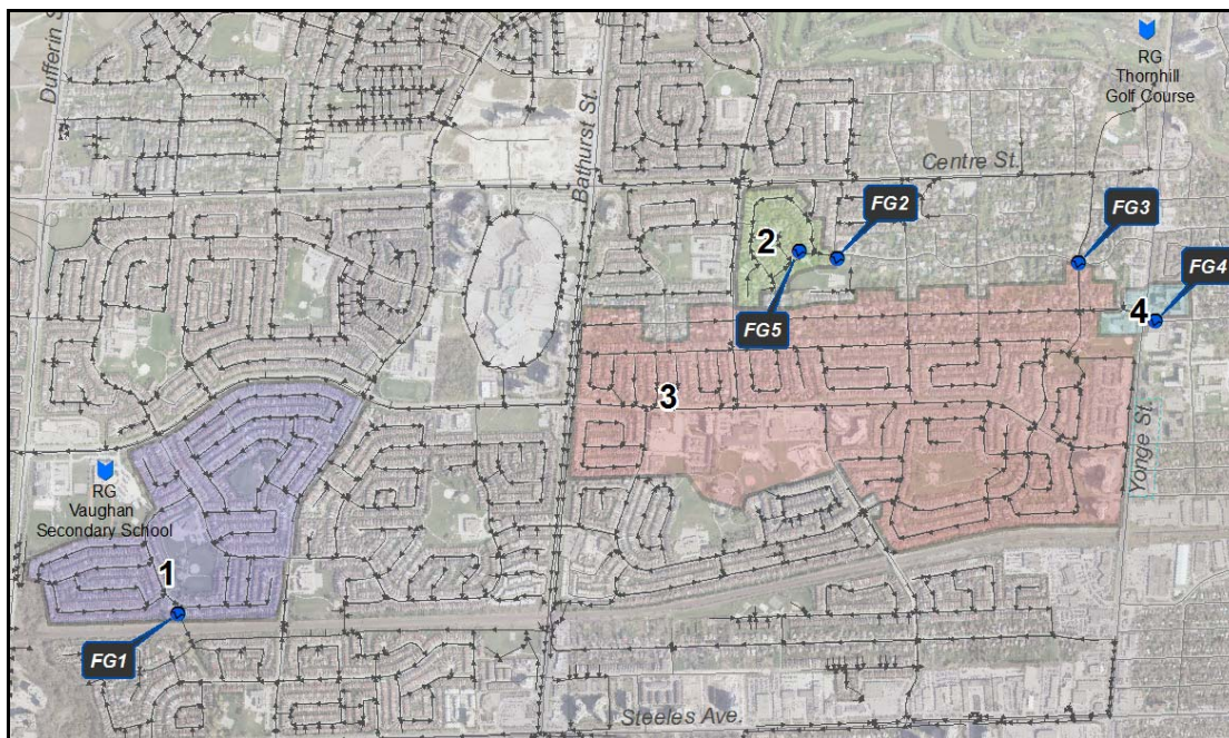
Figure 1-1 Rain Gauge and Flow Monitoring Location Map
