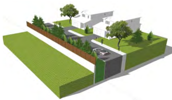
View AA - Existing Condition 2.4 m Wood Privacy Fence with Gravel Retaining Wall along VHCP Property Line
