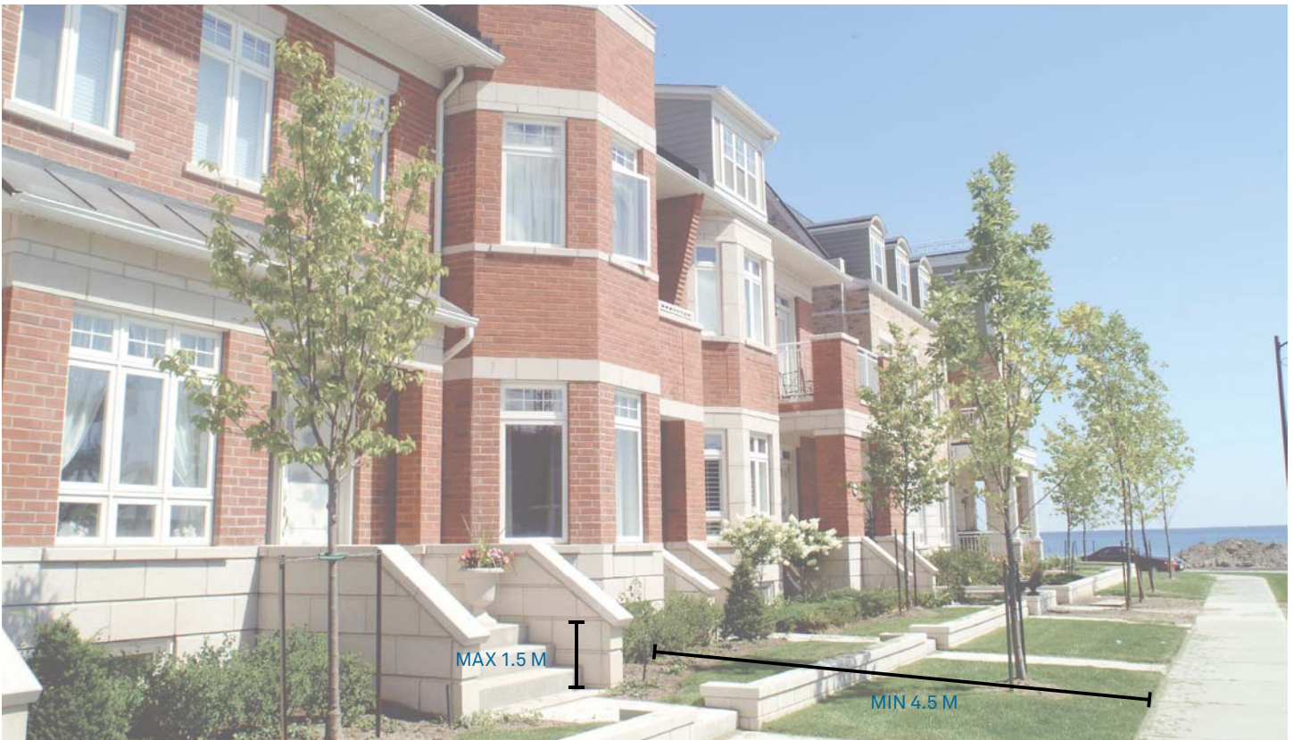
Entrances to individual units should be no more than 1.5 metres above existing grade and incorporate a 4.5 metre front yard setback. (Image Credit: Brook McIlroy).
