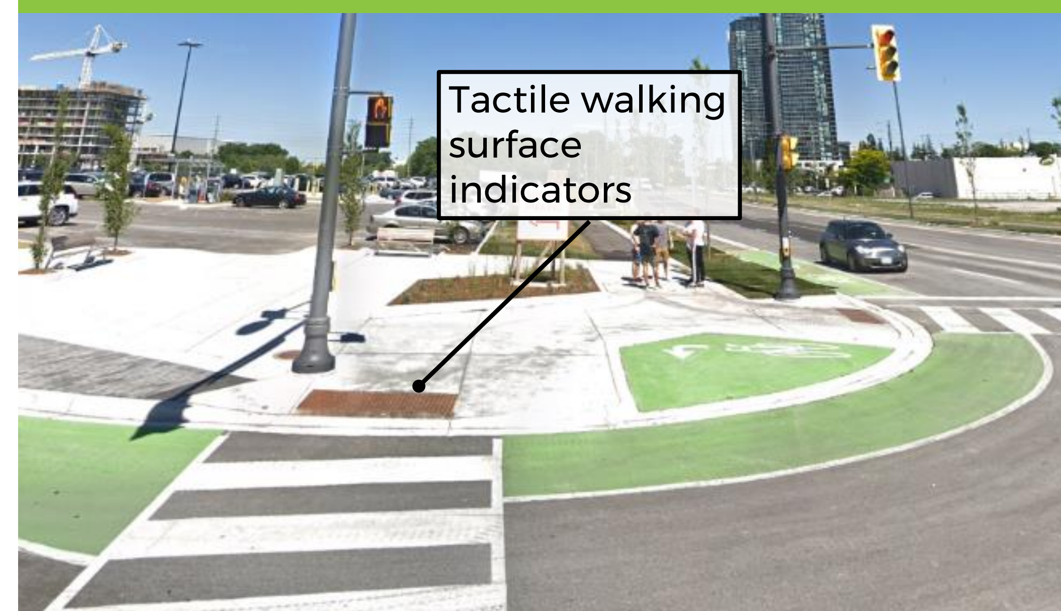
Intersection with tactile walking surface indicators
