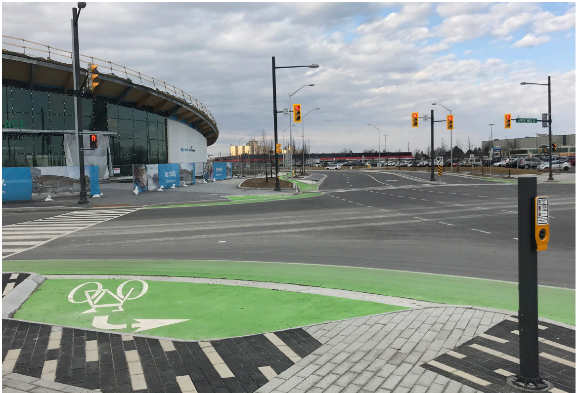
Bike Box at Millway Avenue and Applemill Road within the Vaughan Metropolitan Centre
