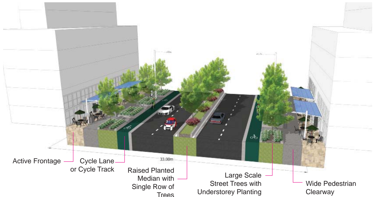
Figure 5.7: Major Collector (Typical Mid-block)
