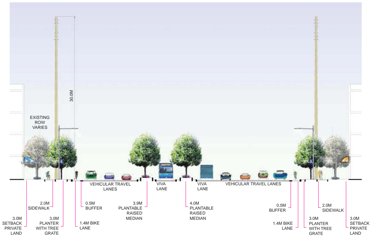
Figure 5.44: Highway 7 at Edgeley Boulevard (Typical Mid-block)
