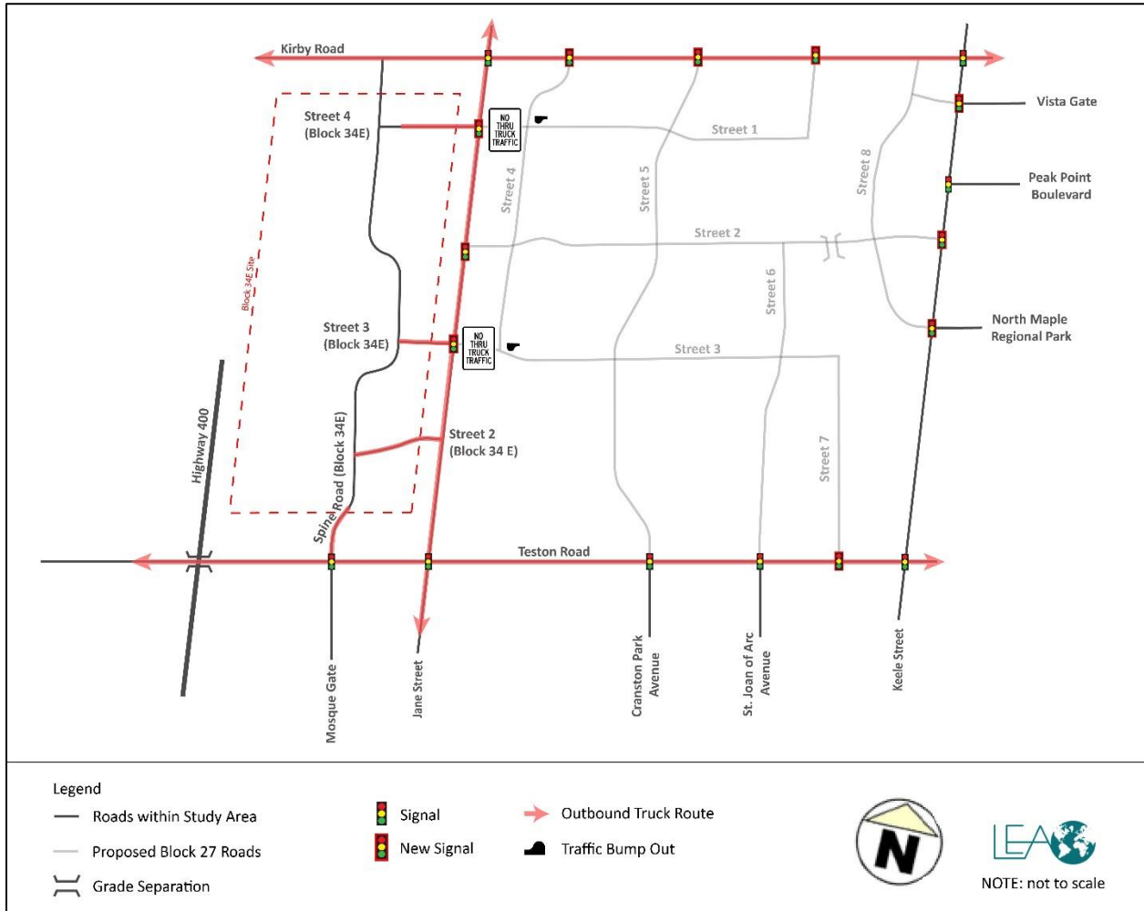
Figure 8-2: Proposed Truck Routing and Mitigation Measures (Outbound Traffic)
