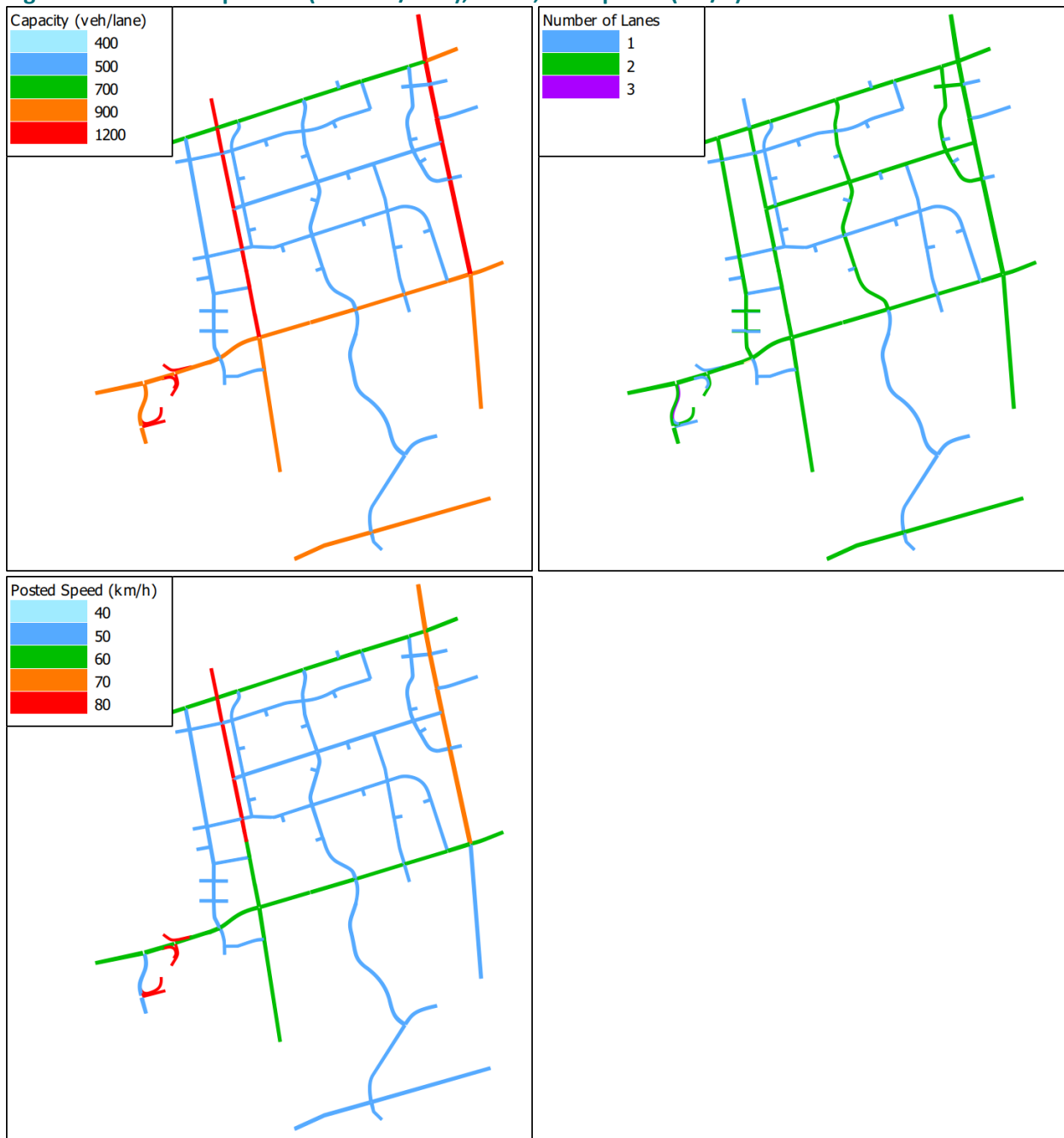
Figure 3-1: Future Capacities (vehicles/lane), Lanes, and Speeds (km/h)
