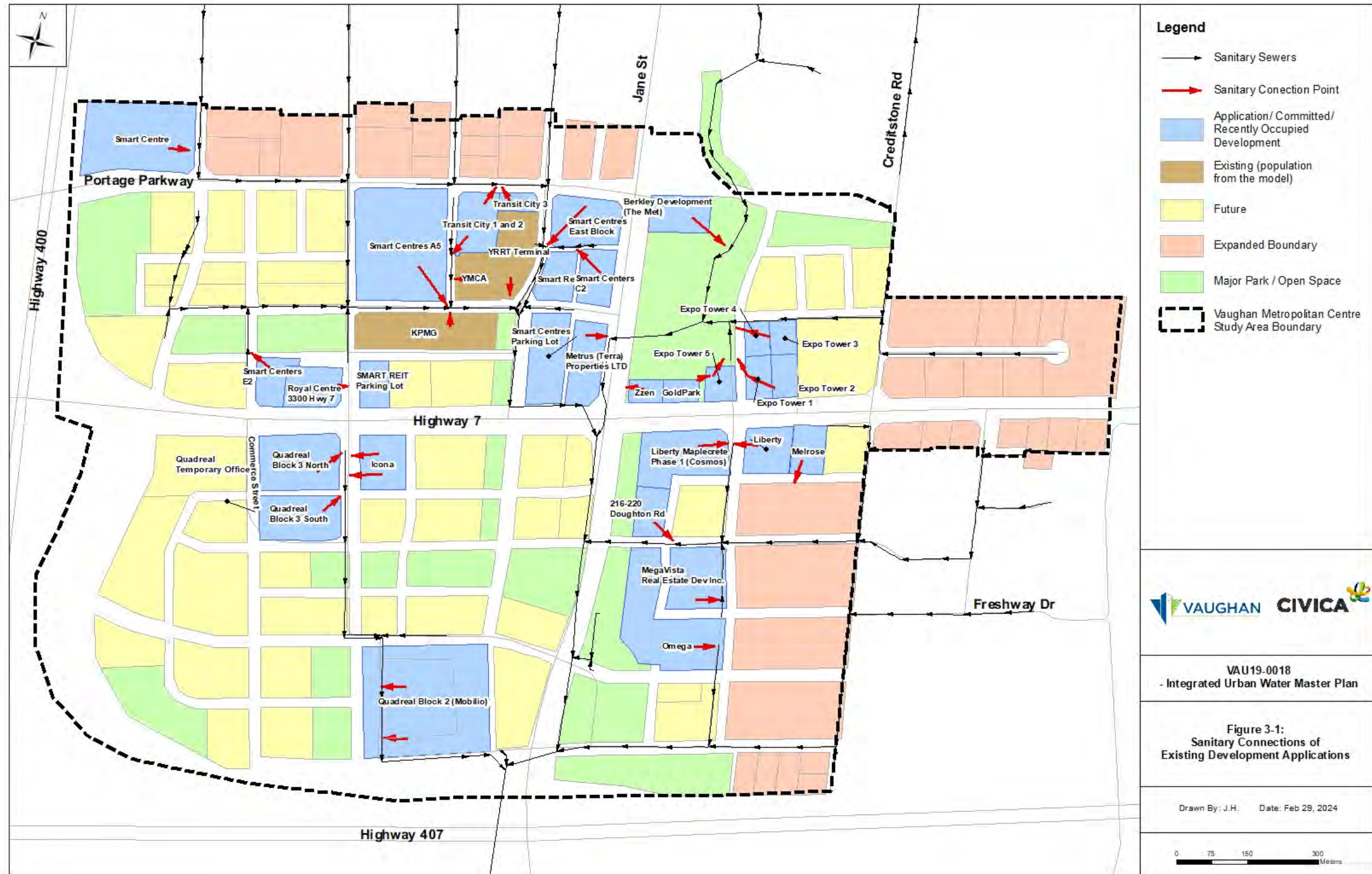
Figure 3-1: Sanitary Connections of Existing Development Applications
