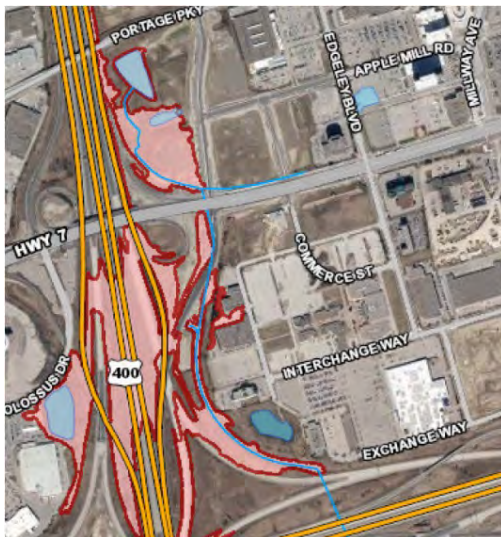
Figure 1-4 Extent of Floodplain through the VMC Northwest and Southwest Quadrants under the Regional Event
