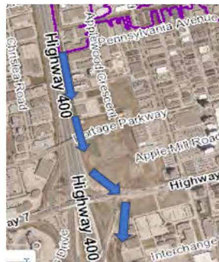
Figure 1-5 Flow path of Black Creek Spill under the 350 year and Regional storm events
