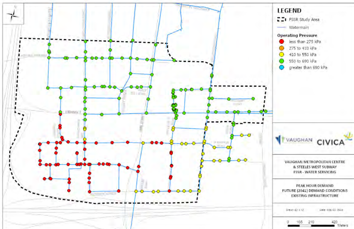
Figure 1-7: Pressures, Future (2041) PHD Conditions, Existing Water Servicing
